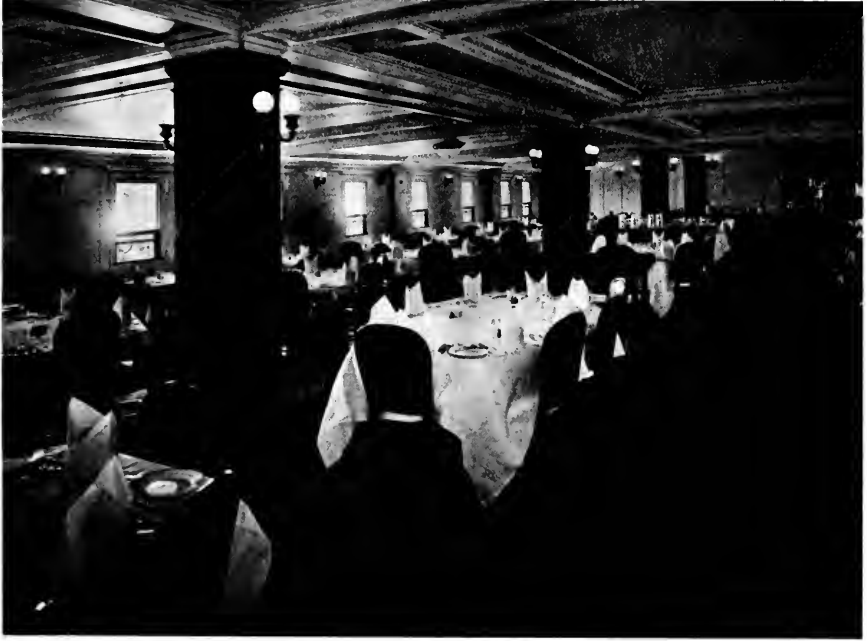
One feature of the dining salon is the wide spacing of tables, and the effect of spaciousness has been increased by the use of "Nevasplit" panels, enabling the very large flat ceiling panels shown in this picture.
